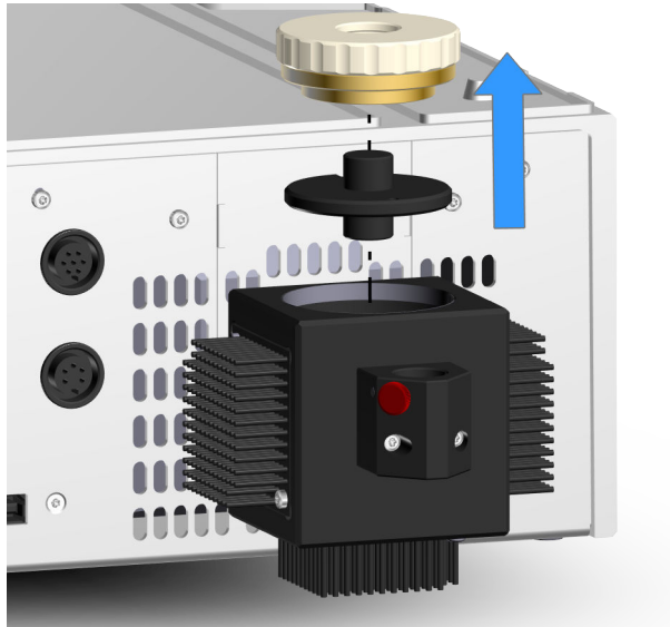
Figure 17 Removing the socket cap for the UV lamp
