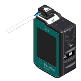
Slide the SERS paper substrate, **printed side** down, into the slot on the side of the attachment. Insert the strip until resistance is met. The attachment accommodates the strip up to the optimal depth.
