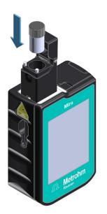
Open the Vial Holder and insert a vial to measure its contents.
