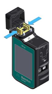
Open the Tablet Holder. Push the levers and position the sample in the middle.
