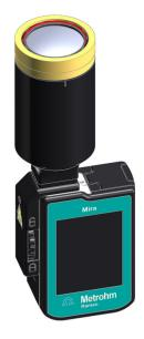
Manually adjust the adjustment ring to the desired Stand-off distance and perform the measurement.
