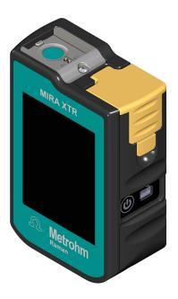
Push the lid downwards until it lock release mechanism engages.
