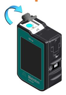
Attach the Smart Tip by engaging the bottom left corner of the attachment into the left edge of the mounting point. Rotate the attachment into position.
