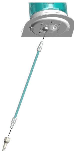
Figure 10 Installing a connection to waste
