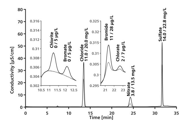
The grey chromatogram corresponds to the sample directly injected while the black chromatogram corresponds to the sample spiked with 10 mg/L chloride, nitrate, and sulfate, 100  $\mu$ g/L fluoride, 20  $\mu$ g/L nitrite and bromide, and 5  $\mu$ g/L chlorite, bromate, and chlorate.
