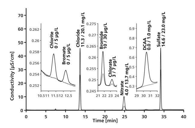
The grey chromatogram corresponds to the sample directly injected while the black chromatogram corresponds to the sample spiked with 10 mg/L chloride, nitrate, and sulfate, 1 mg/L dichloroacetate, 100  $\mu$ g/L fluoride, 20  $\mu$ g/L nitrite and bromide, and 5  $\mu$ g/L chlorite, bromate, and chlorate.
