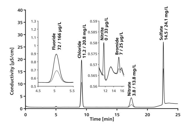
The grey chromatogram corresponds to the mineral water sample directly injected while the black chromatogram corresponds to the same sample spiked with 10 mg/L chloride, nitrate, and sulfate, 100  $\mu$ g/L fluoride, and 20  $\mu$ g/L nitrite and bromide.
