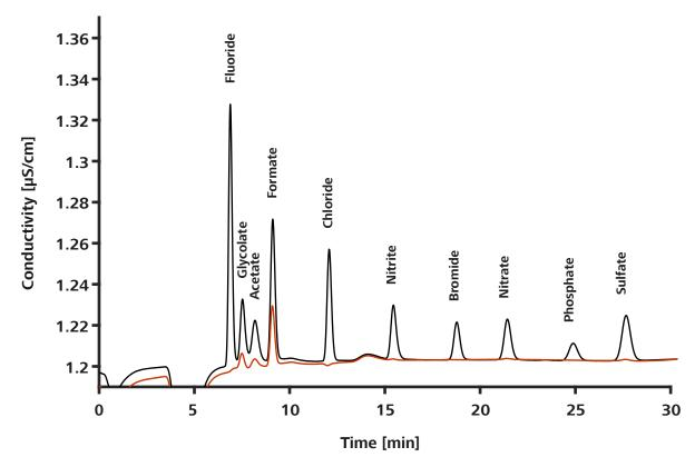
The red chromatogram corresponds to boiler feed water with 4.0 mg/L ethanolamine and 0.4 mg/L ammonia. The black chromatogram shows the same sample to which 2  $\mu$ g/L of the standard anions and of the organic acids glycolate, acetate and formate were added.
