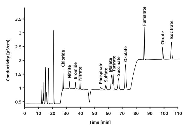
In the back part of the chromatogram, higher eluent concentrations are used to elute the multivalent analytes. Organic acids are also dissolved after sulfate.
