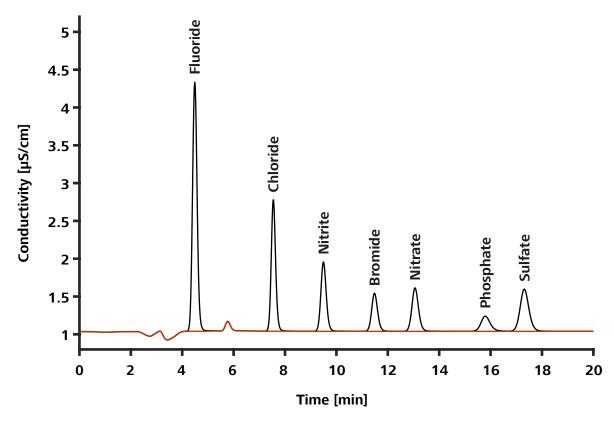
The red chromatogram corresponds to the direct injection of the ethanol sample onto the column. The Metrosep A Supp 19 - 150/4.0 is inert when injecting organic solvents, such as ethanol. The black chromatogram
