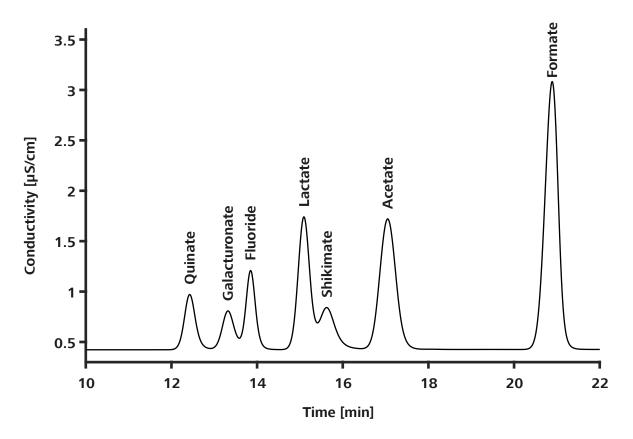
In addition to the determination of standard anions, the Metrosep A Supp 19 - 250/4.0 is particularly suitable for the determination of low-molecular-weight organic acids. Quinate, galacturonate, fluoride, lactate, shikimate, acetate and formate can be reliably resolved in the front part of the chromatogram with gradient elution. The column can thus be of excellent use for determinations in food samples.
