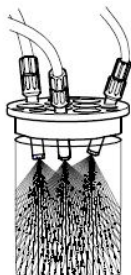
Figure 18: Installation of rinsing nozzles
