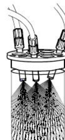
Figure 18: Installation of rinsing nozzles
