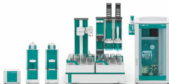
Figure 9: Complete TitrIC flex I setup
