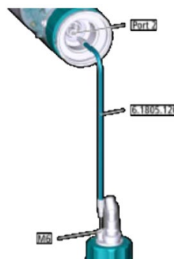
Figure 6: Dosino connections for regeneration
