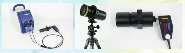
Replacing the shaft of a BAC102 probe with an RTS20x series zoom lens allows for stand-off Raman measurement. The lenses have adjustable working distances making them suitable for different environments such as measurement inside thick-walled glass reactors or non-contact high temperature, high pressure measurements.
