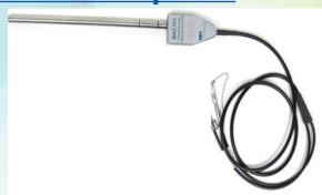
The industrial immersion probes on B&W Tek's laboratory Raman instruments feature a stainless steel probe body along with a stainless steel or hastelloy probe shaft. They are immersible in liquids, slurries, powders, and solids under pressure up to 4000 psi and temperatures up to 300 °C for hastelloy (200 °C for stainless steel). Fiber cable length 1.5m.
