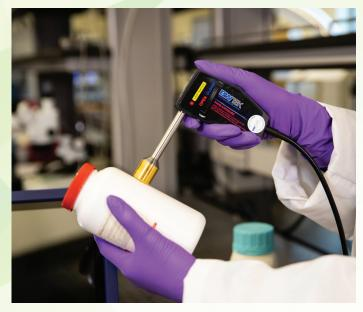
B&W Tek also offers see-through probe with increased penetration depth that can be used with our i-Raman Prime 785 or i-Raman EX (1064 nm) system to identify material through opaque packaging when used with our BWID software. With a large 4 mm diameter measurement area, bulk property measurements of heterogeneous samples can be made.
