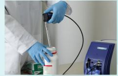
The standard probes on B&W Tek's laboratory Raman instruments (model BAC102-xxx) come with standard aluminum shafts that are 3" (76.2 mm) in length with a diameter of 0.371" (9.42 mm), operable up to 80°C for non-immersive use (model RSS100-xxx). In addition, the shafts on these probes are user-replaceable, giving the flexibility to adapt to different working environments.
