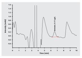
0.1 µg/L bromate spiked in tap water sample, column: Metrosep A Supp 16 - 150/4.0, eluent: 100 mmol/L  $H_2SO_{ar}$ 19.3 µmol/L ammonium heptamolybdate, flow 0.8 mL/min, 45 °C, post-column reagent: 0.27 mmol/L KI, flow 0.15 mL/min sample volume 1200 µL, wavelength 352 nm.
