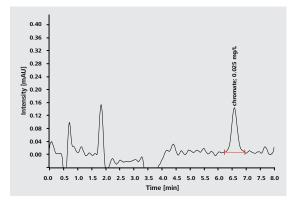
Chromate 0.025 µg/L, column: Metrosep A Supp 17 - 100/4.0, eluent: 70 mmol/L NH<sub>4</sub>NO<sub>3</sub>, 7.0 mmol/L NaOH, flow 0.7 mL/min, 45 °C, postcolumn reagent: 2 mmol/L 1.5 - diphenylcarbazide, 10% ethanol, 0.5 mol/L sulphuric acid, flow 0.22 mL/min, sample volume 1.325 mL, wavelength 538 nm.
