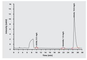
Nitrite ((0.5 mg/L), bromide (1.0 mg/L) and nitrate (10 mg/L) in artificial sea water, (28 g/L NaCl), column: Metrosep A Supp 10 - 250/4.0, eluent: 5.0 mmol/L Na<sub>2</sub>CO<sub>3</sub>, 5.0 mmol/L NaHCO<sub>3</sub>, flow 1.0 mL/min, 40 °C, chemical suppression, sample volume 10  $\mu$ L, wavelength 218 nm.
