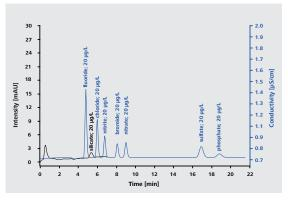
Silicate next to standard anions (0.02 mg/L), column: Metrosep A Supp 17 - 150/4.0, eluent: 5.0 mmol/L Na<sub>2</sub>CO<sub>3</sub>, 0.2 mmol/L NaHCO<sub>3</sub>, flow 0.6 mL/min, 45 °C, postcolumn reagent: 20 mmol/L Na<sub>2</sub>MoO<sub>4</sub>, 200 mmol/L HNO<sub>3</sub>, flow 0.3 mL/min, sample volume 200  $\mu$ L, wavelength 346 nm.
