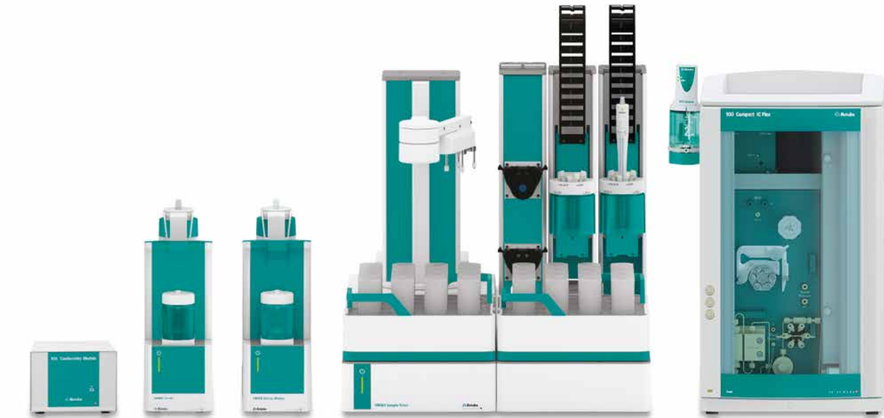
TitriC Flex I – the fully automated system for direct measurement of temperature, conductivity and pH value, the titrimetric determination of the p and m values, calcium, and magnesium. Anions are determined simultaneously by ion chromatography after passing through Inline Ultrafiltration.
