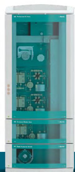
940 Professional IC Vario with conductivity and amperometric detection. The high-pressure gradient system is extendable with the 942 Extension Modules to up to a quaternary high-pressure gradient system or the 941 Eluent Production Module.
