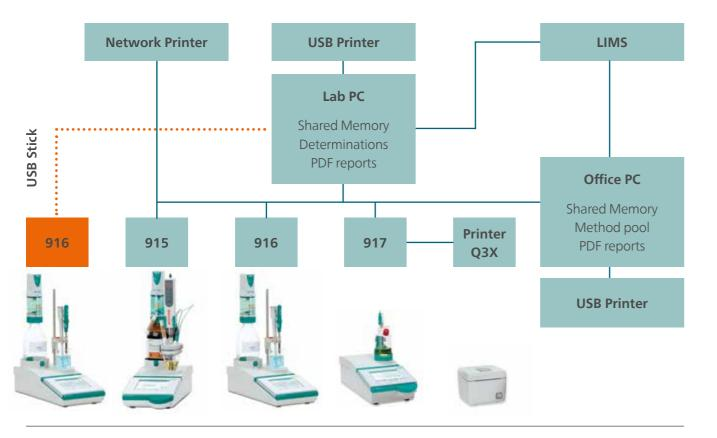
Integrate the Ti-Touch Family in your networked laboratory: automatically export PDF reports/determination files to your LIMS on your lab/office Computer, print on local or network printers, and share titration methods from a centralized network directory. Even data from instruments not connected to the network can be transferred via manual export to a USB memory stick.
