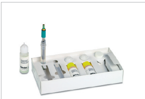
3. Immerse electrode in the cleaning solution beyond diaphragm and let the solution take its effect
