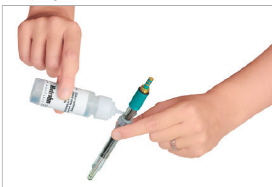
5. Rinse electrolyte chamber with electrolyte and refill it
