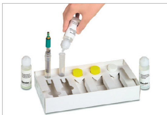
6. Exchange storage solution in the electrode storage vessel
