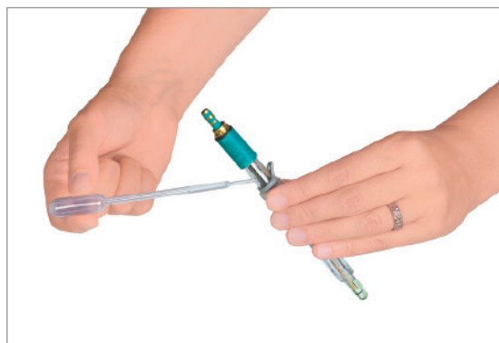
4. Empty electrolyte chamber
