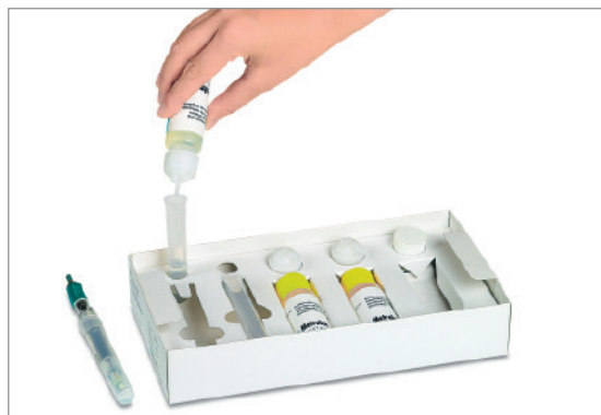
2. Fill in cleaning solution
