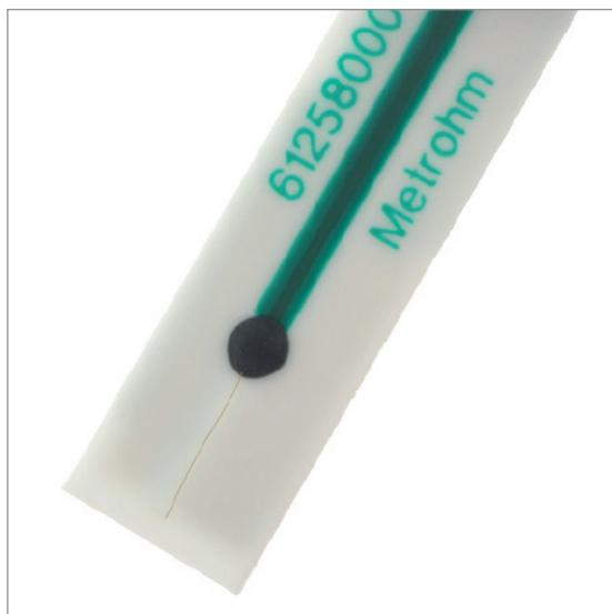
As with any electrode, the performance of the scTRACE Gold deteriorates as more and more determinations are performed. However, the practical plug-in design means that only the cost-efficient sensor has to be replaced, so regular replacement is not a problem. This ensures reliable results at all times. The electrode shaft can further be used.
