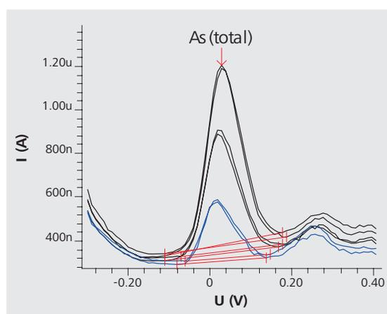
$\beta(\text{As}(\text{total})) = 4.8 \text{ } \mu\text{g/L}$  in mineral water with two standard additions
