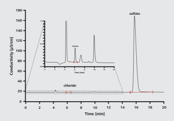
Chromatogram (left): Determination of halogens and sulfur in certified polyethylene pellets ERM-EC681k: chloride: 102.4%, bromide 95.4%, sulfur 100.3%. Injection volume 20  $\mu$ L
