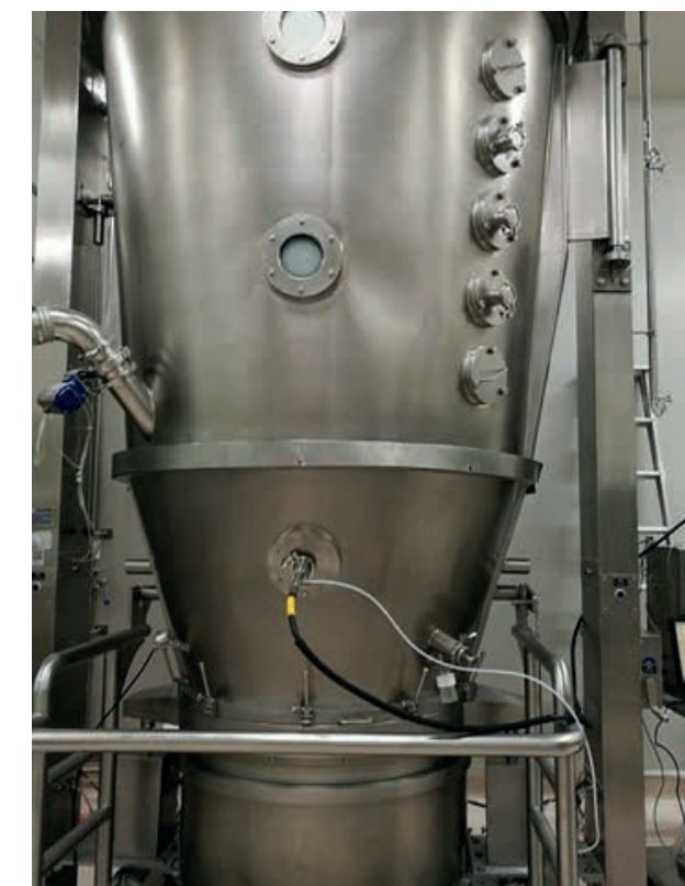
Spoon probe implemented in a dryer.
