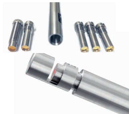
Top: Single fiber transmittance probe with a set of mirrors for defined OPL (left to right): 0.5 mm, 1 mm, 2 mm, 5 mm, 10mm. Bottom: Microbundle fiber transmittance probe with adjustable mirror.
