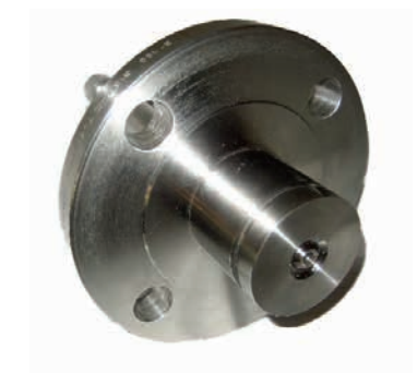
Diffuse reflectance probe.
