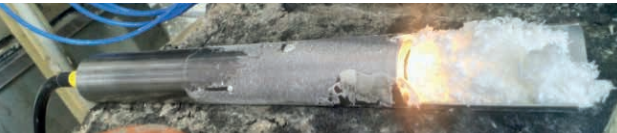
Example of non-contact probe inserted in an outer sleeve for fluffy samples.
