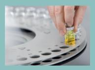
Heating vial by vial, the water contained in the samples is evaporated. A constant stream of an inert carrier gas is used to bring the water fraction into the titration cell, where it is determined. The sample matrix stays in the vials, which are simply disposed of after the titration.
