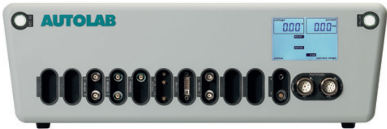
PGSTAT302N with ADC10M, SCAN250, FRA32M, and ECI10M modules.
