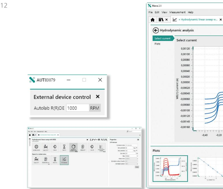
The NOVA software is used to control all Autolab potentiostat/galvanostat and accessories connected to it. It provides a simple and modern interface to all electrochemical experiments and comes with an extensive library of methods suitable for a wide range of applications.
