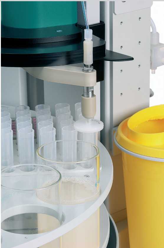
Fully automated filtration: The 815 Robotic Filtration Soliprep filters out residual solid matter from the homogenized sample. What remains is a clear filtrate that can be either injected directly into an analyzer or subjected to further dilution.
