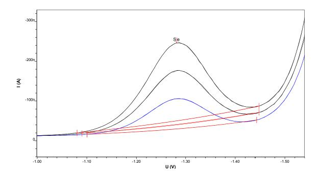
Selenite can be determined in electrolyte solutions used in production of copper indium gallium selenide solar cells – also called CIGS cells – for the electrodeposition of the CIGS absorber layer.
