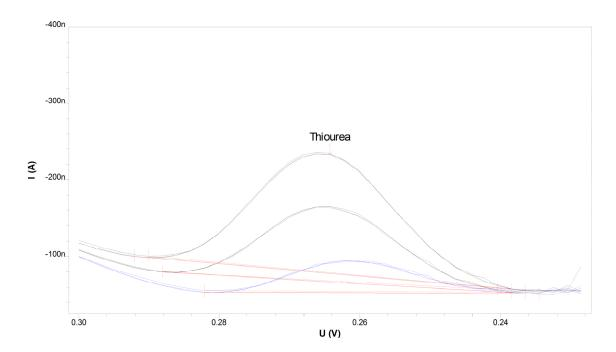
Copper is produced using an electrolysis procedure. Thiourea is added to the copper electrolyte to optimize plating efficiency. With voltammetry thiourea can easily be determined in highly concentrated copper electrolyte solutions containing sulfuric acid and small amounts of chloride.
