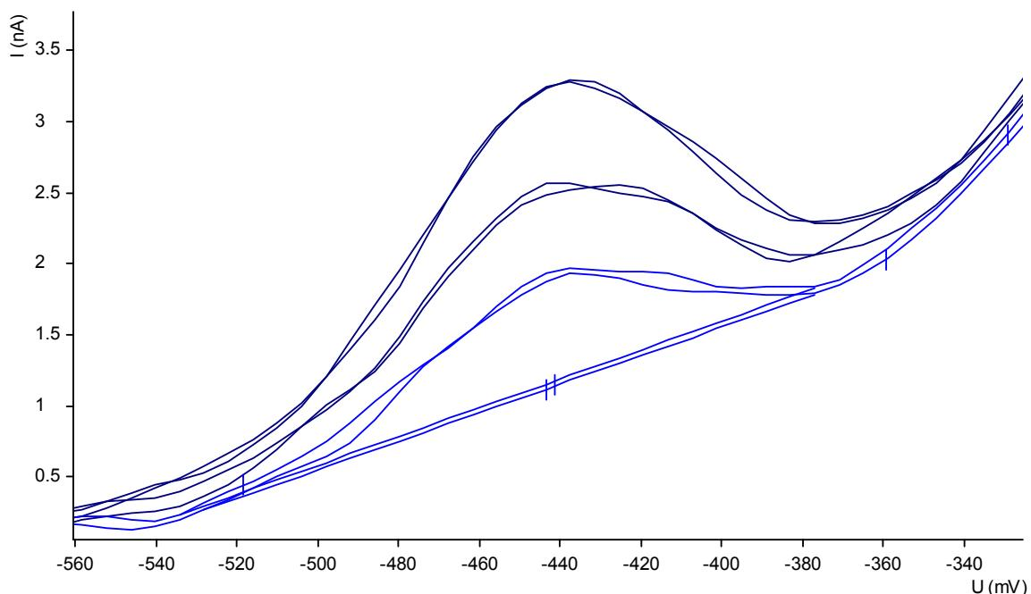
Thallium in waste water is determined in acetate buffer in presence of EDTA by anodic stripping voltammetry (ASV). Samples with organic substances have to undergo UV digestion before analysis.
