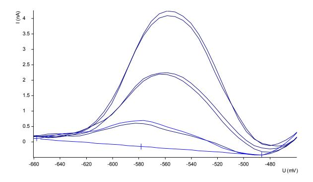
Tin can be determined in waste water by anodic stripping voltammetry (ASV) in oxalate buffer after addition of methylene blue. Samples with organic substances have to undergo UV digestion before analysis. Samples with higher concentrations of metals can be diluted before digestion.
