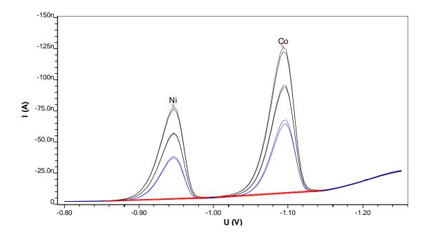
The determination of nickel and cobalt in waste water samples can be carried out using adsorptive stripping voltammetry after UV digestion of the sample according to DIN 38406 part 16.
