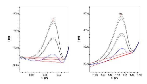
For the determination of heavy metals in wine, UV digestion is required to mineralize the sample. The determination of platinum and rhodium is carried out with adsorptive stripping voltammetry (AdSV) at the HMDE.
