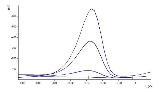
For the determination of nickel in white wine, UV digestion is required to mineralize the sample. The determination is done by adsorptive stripping voltammetry (AdSV) at the HMDE in ammonia buffer with dimethylglyoxime (DMG).
