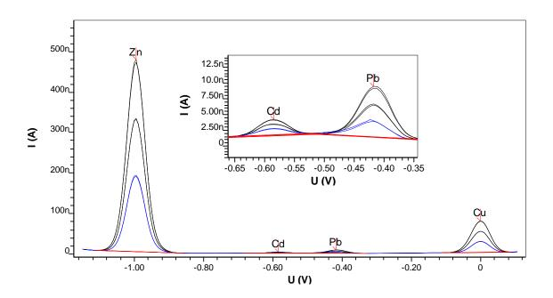
Zinc, cadmium, lead, and copper can be determined in waste water samples after UV digestion by anodic stripping voltammetry according to DIN 38406 part 16.
