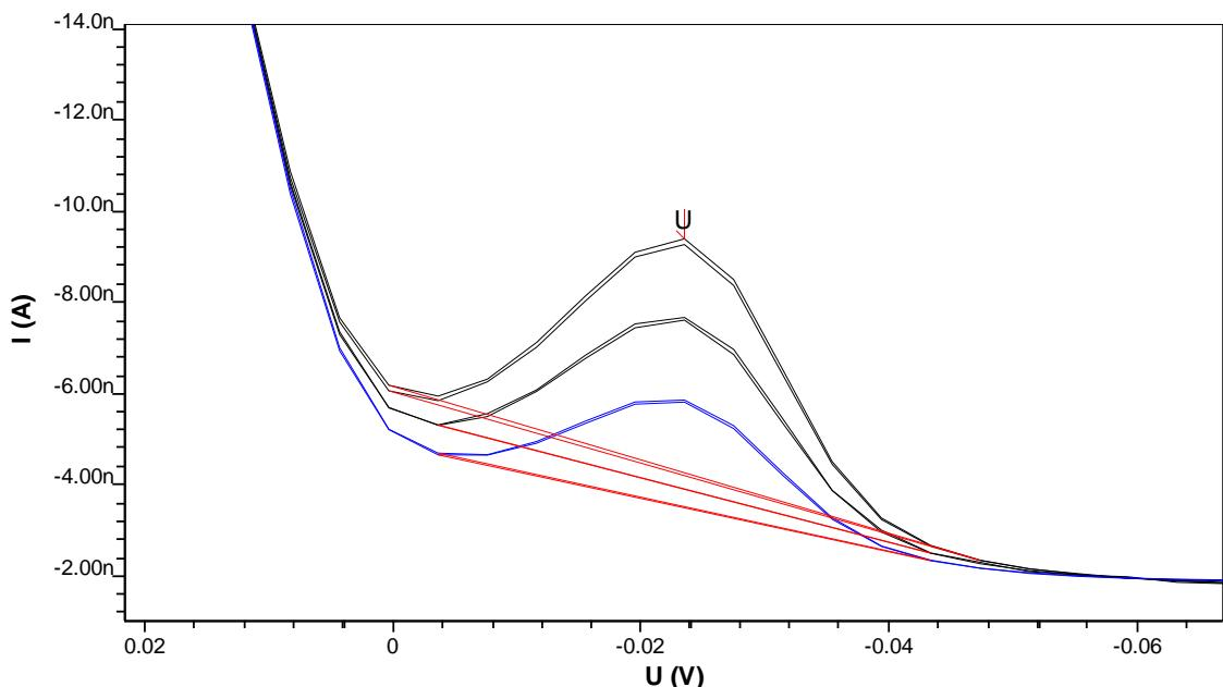
Uranium can be determined in drinking water by adsorptive stripping voltammetry (AdSV) at the hanging mercury drop electrode (HMDE). Chloranilic acid is used as complexing agent.
