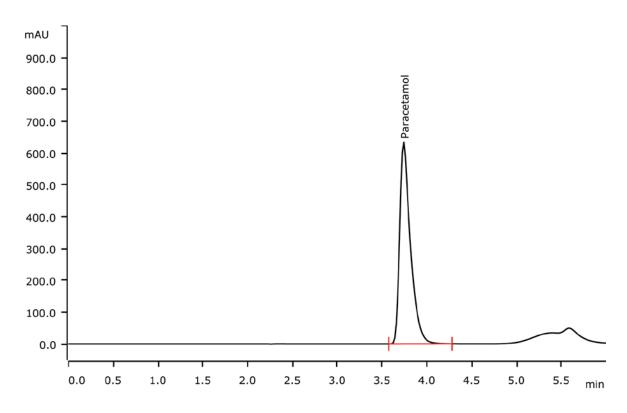
Paracetamol is a very effective analgesic and antipyretic drug. Using the presented sample preparation, its determination in tablets by reversed-phase chromatography and UV detection is straightforward. The fully automated 815 Robotic Soliprep for LC takes over everything, starting from the tablet dissolution, homogenizing and filtration to the injection with a 250 nL internal loop.
