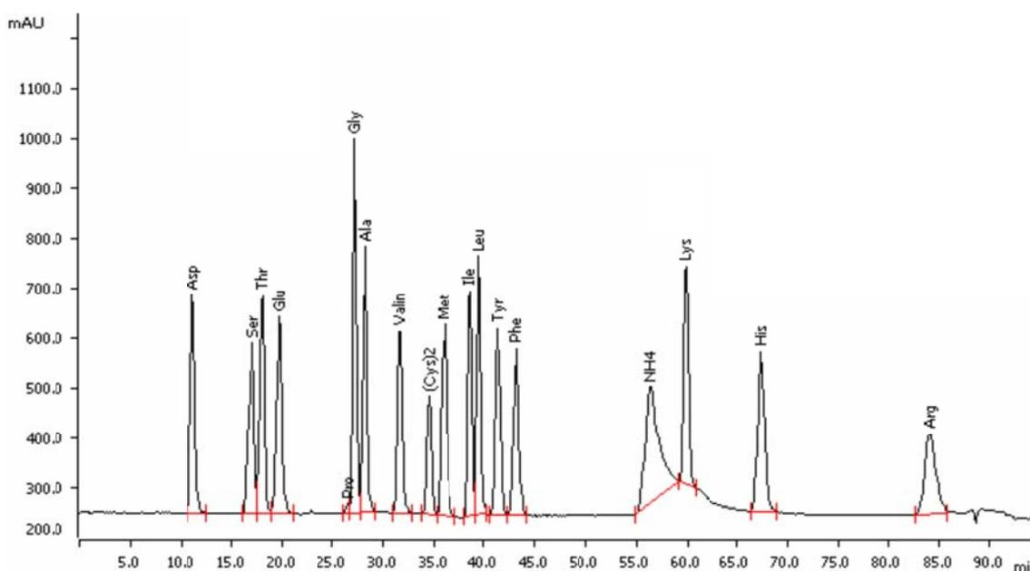
The determination of amino acid is an important task in pharmaceutical and biochemical applications. A binary gradient separates in this example 17 amino acids of a commercially available standard solution. The post-column reaction with ninhydrin requires a temperature of 120 °C, while the samples need to be cooled for stability.
