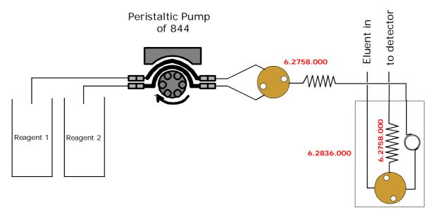
It is important to replace the PTFE mixing coil of the Post Column Reactor (6.2836.000) by a PEEK mixing coil (6.2758.000). Iodine can diffuse through PTFE and this will lead to severe peak tailing.
