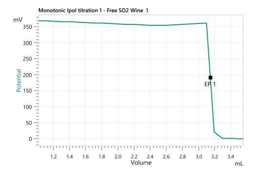
The analysis of the reductants, free and total sulfurous acid, pH and total acidity of wine can be performed fully automated on an OMNIS system based on the directive OIV-MA-AS323-04B. OIV-MA-AS313-01 and OIV-MA-AS313-15.
