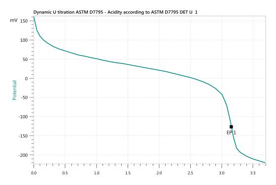
Denatured fuel ethanol may contain additives such as corrosion inhibitors and detergents as well as contaminants from manufacturing that can affect the acidity of produced ethanol fuel. An increased acid content in solvents could lead to a variety of problems like a shorter storage stability or chemical corrosion.
