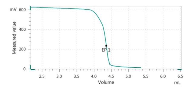
Vitamin C is an important antioxidant included in milk powder. The double Auring electrode provides an excellent titration curve when using 2,6-dichlorophenolindophenol (DPIP) as titrant and is easy to clean.
