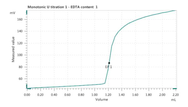
Complexing agents like EDTA are used in soaps and other detergents for the removal of undesired metal ions and for lowering the water hardness. The EDTA content in soaps and detergents can be determined by potentiometric titration using the Cu-ISE for indication and cupric sulfate as titrant.
