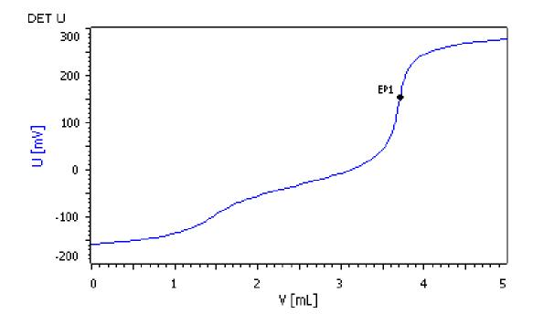
The basicity and the CPR (controlled polymerization rate) are very important parameters for the quality of polyols used in polyurethane production. The knowledge of these values is crucial to prevent gelation during handling in the production. In this Application Note their determination by automated, potentiometric titration according to ISO 14899 is described.
