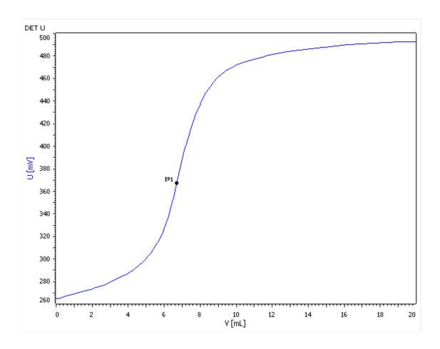
Alkyl glycosides, alkyl maltosides, and compounds with polyoxyethylene (POE) groups belong to nonionic surfactants. These surfactants can be analyzed with a standard titration against TEGO®trant after derivatization (i.e., sulfonation).
