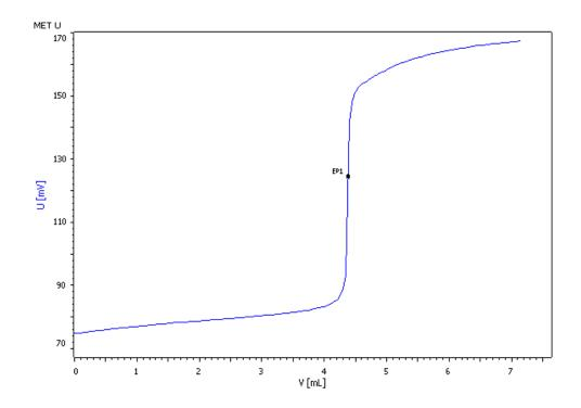
Thorium is determined at pH 4.9 by titration with EDTA. To visualize the equivalence point, xylenol orange is used as indicator. The equivalence point is detected with the Optrode at a wavelength of 574 nm.
