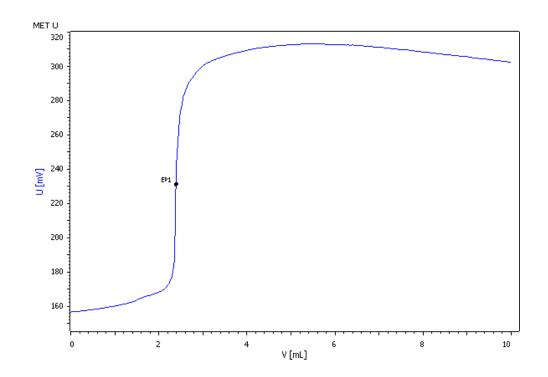
Zirconium can be determined in acidic aqueous solutions (buffer pH 1) by direct titration with EDTA. Eriochrome cyanine R is used as indicator. For equivalence point indication, the Optrode is used at a wavelength of 520 nm.
