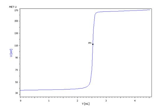
Tin forms very stable complexes with EDTA in its divalent and tetravalent form. In alkaline media, tin forms hydroxo complexes for which reason tin is titrated in acidic medium (pH 2.1). Xylenol orange is used as indicator; the equivalence point is detected with the Optrode at a wavelength of 574 nm.
