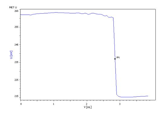
Mercury can be determined in alkaline media by back-titration with zinc sulfate using eriochrome black T as indicator and the Optrode at a wavelength of 502 nm for indication.
