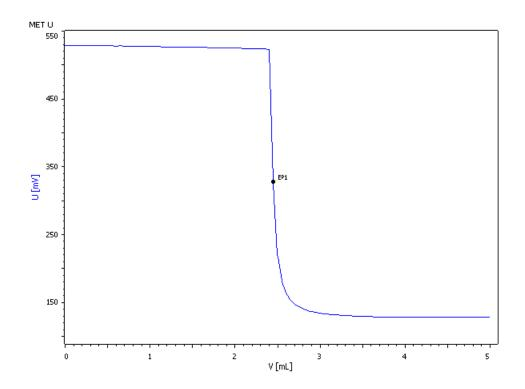
Lead is determined at pH 4 to 5 by back-titration with zinc sulfate. To visualize the equivalence point, xylenol orange is used as indicator, and the equivalence point is detected with the Optrode at a wavelength of 574 nm.
