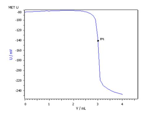
Cadmium can be analyzed using the Cu ISE. A small amount of Cu-EDTA complex thereby acts as indicator as the Cu ISE itself is not sensitive for cadmium.
