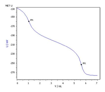
This application note describes the automated determination of sulfate using the combined Ca ISE as sensor. The sulfate is precipitated with an excess of barium, which is then back-titrated with a standard EGTA solution.
