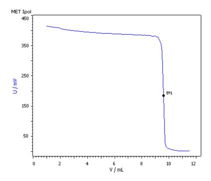
This application note describes the iodometric, bivoltametric determination of ascorbic acid in orange juice using the Double Pt-sheet electrode
