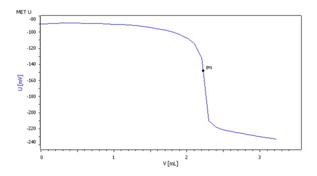
This Application Note describes the fully automated complexometric determination of zinc(II) in aqueous solutions with a copper ion-selective electrode and the MATi 07 system.
