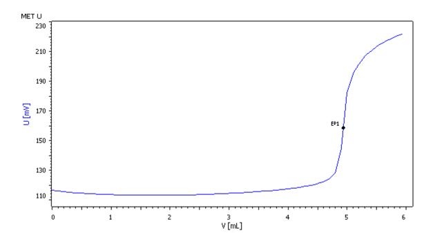
This Application Note describes the fully automated complexometric determination of iron in cement (digested) with a copper ion-selective electrode and the MATi 07 system.
