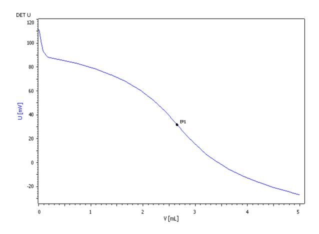
The automated system determines the chloride content in all kind of water samples. The high degree of automation (e.g., automated acid addition, as well as automated titer determination) minimizes errors and guarantees an outstanding reproducibility.
