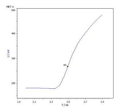
The Application Note describes the photometric determination of sulfate using the Optrode (610 nm). Sulfate is titrated with a lead nitrate solution using dithizone as indicator.
